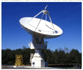
Twice the diameter of the world's largest visible-light telescope, this telescope, once refurbished, will be available for use through Skynet's web page and will be as easy to use as Skynet's visible-light telescopes. Furthermore, one of its capabilities will be 21-cm spectroscopy.
